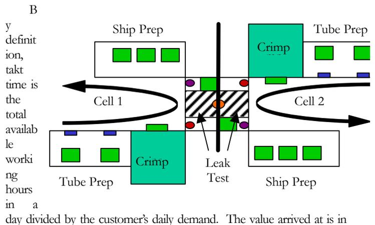
units of time and tells the manufacturer how often a customer needs a part and thus how often to produce. While the takt time calculation is similar to determining belt rate, it is a more integral part of the cell design since a primary design goal of an overall lean system is to match production pace with customer demand (i.e. never under- or overproduce).
