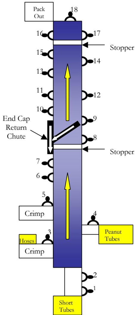
Figure 2. Layout of the assembly line
