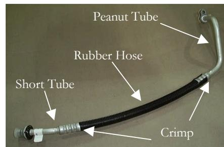
Figure 1: Connector between air conditioning components
