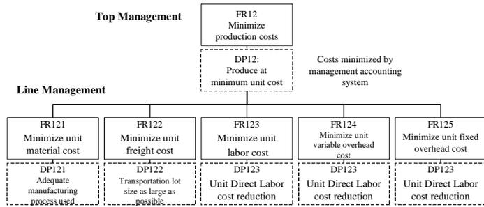
Figure 9. Further Decomposition of Mass Production System – Line Management Level
