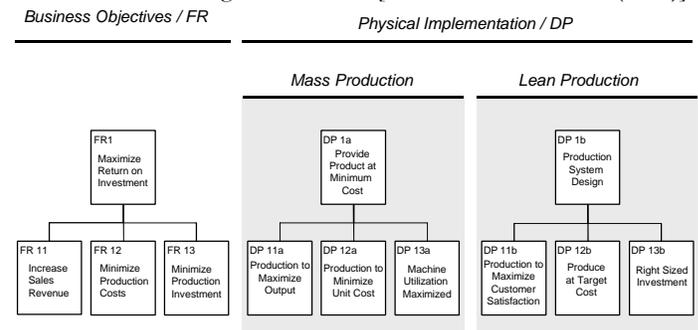
Figure 13. Comparison between Mass Production and Lean Manufacturing system design
