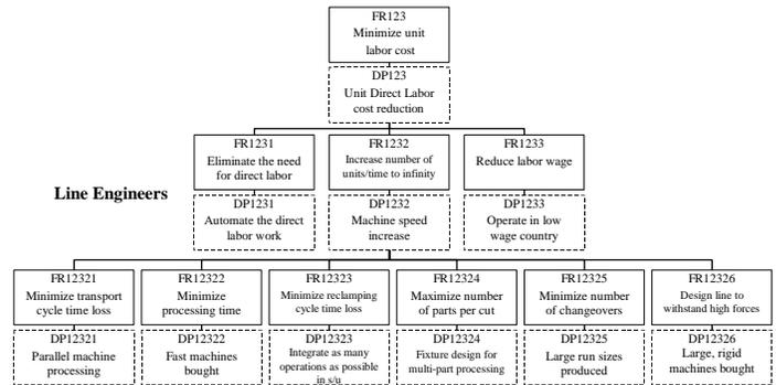
Figure 11. Design Decomposition of Unit Labor Cost Minimization – Line Engineers Level
