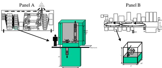
Figure 16. Comparison of Mass and Lean Broach Machine Design [Cochran and Dobbs, 1999]
