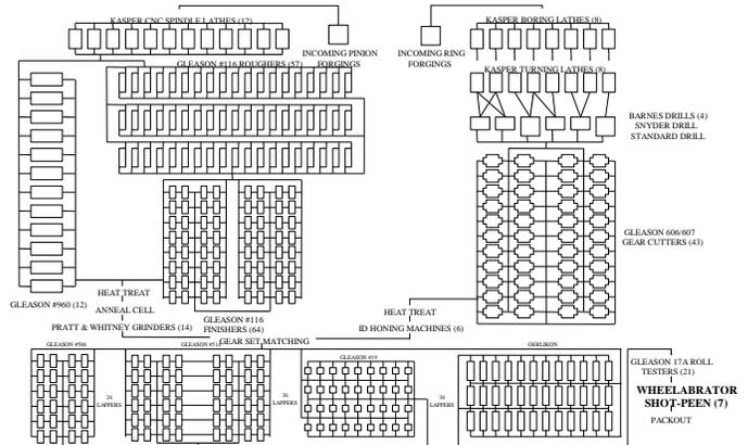
Figure 3. Schematic View of Departmental Mass Production System Layout
